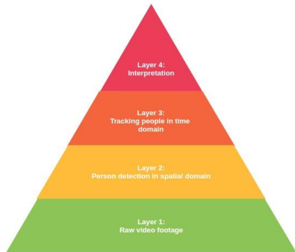
Fig. 3: The abstractedly and dependency of the layered structure of the data could be represented by a pyramid. Every layer is dependent on the layer before, but increases the abstractness of the data.
